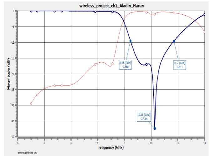
Figure 3. Filter response graph (S11 RED, S12 GREEN)
